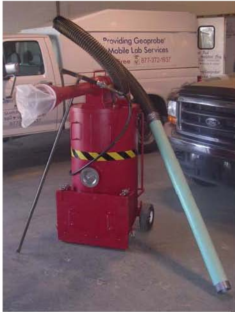
Figure 1: Vacuum Excavation System
